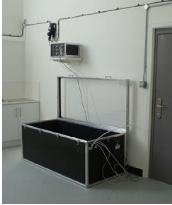
Figure 4 Curing chamber where the specimen is exposed to the gas hardener S6
