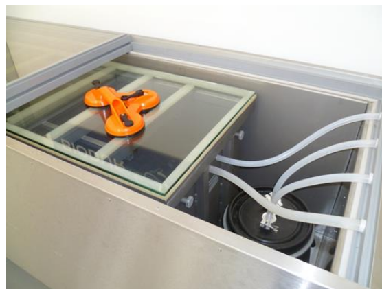
Figure 3 Glass topped vacuum chamber situated with a freezer for impregnation of the S10/S3 polymer mixture
